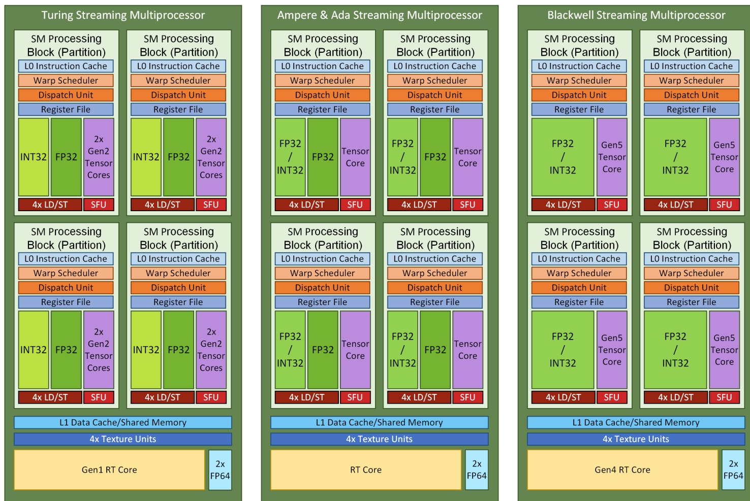
Figure 2: NVIDIA Streaming Multiprocessor architecture for Turing, Ampere/Ada, Blackwell
